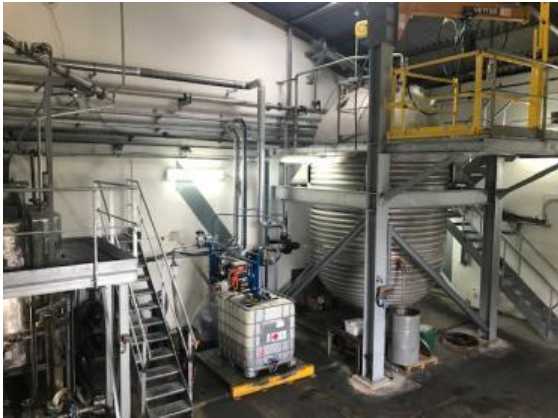
10 m 3 reactor for manufacturing molten resins
