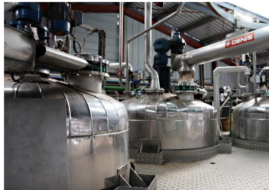
3 x 5,000 litre maceration tanks (steam heating) Characteristics: semi-continuous operation Rate for a simple extract: 30 tonnes of plant materials per week
