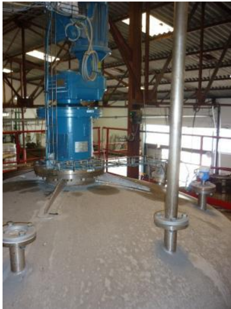
10,000 litre mixer for the manufacture of microemulsions
