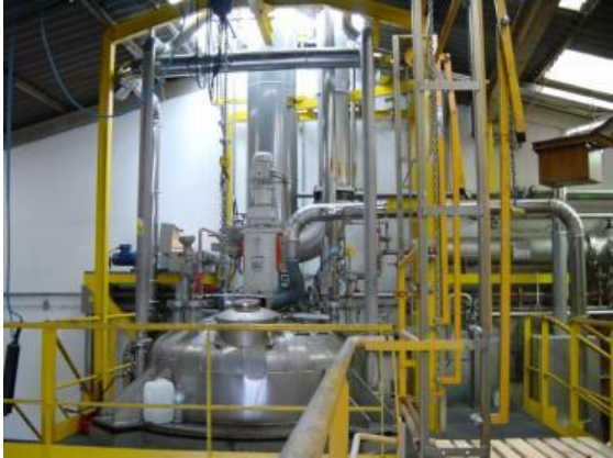
10 m 3 reactor for manufacturing molten resins
